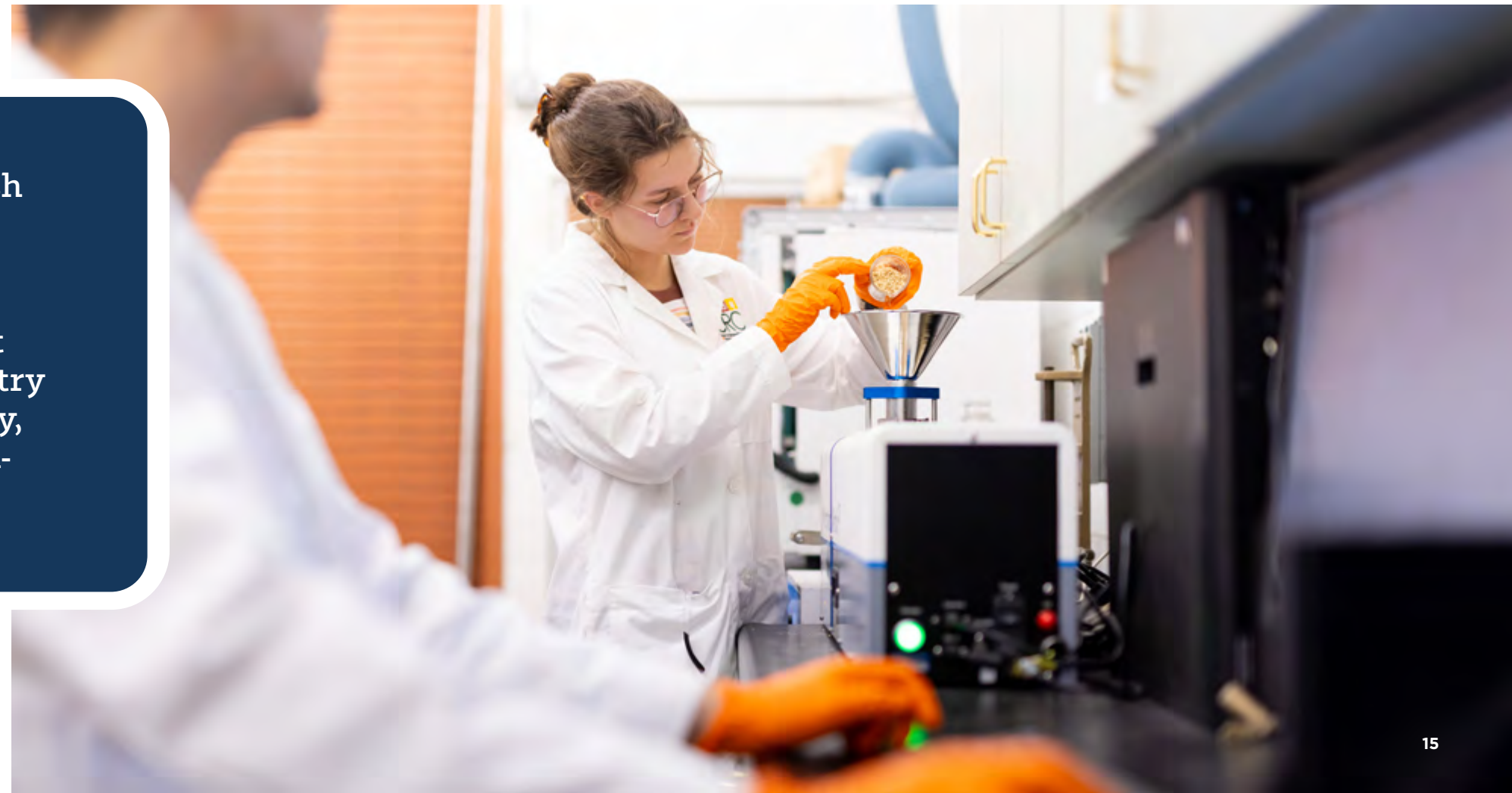
PhD student Yang Li looks at the data as a high school student drops poplar sawdust samples into a particle-sized 3D image analyzer in the Bioenergy and Biofuels Lab on May 8, 2024. Photo by Steven Bridges/University of Tennessee, Knoxville.
